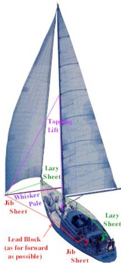
**Do not attempt to retract or telescope a pole under load.** You will not be able to handle any pole under load and can injure yourself. Be sure all sheets are slack before setting, telescoping or taking down a pole.
