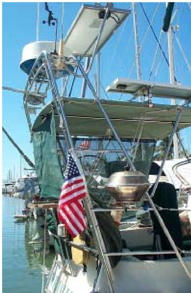
Arch system for solar panels, radar, antennae, and davits
