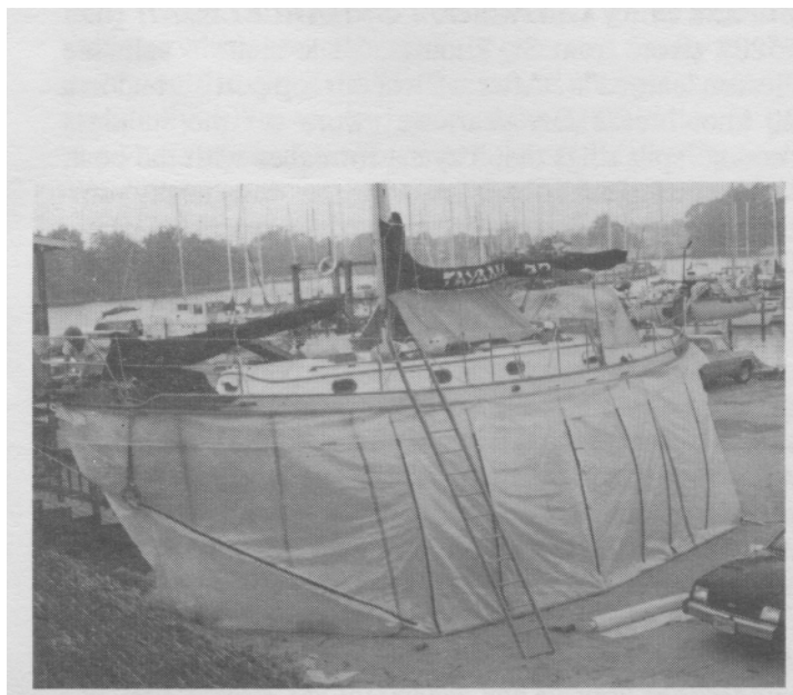
DRYING OUT. Airtight tent built around and under hull, plus heat and dehumidifier aids the drying process.
