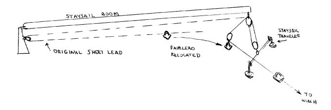
This arrangement has eliminated the compression load on the boom, and the loose sheets hanging up on the dorade vents (one owner lost a cowl vent this way). Incidentally, if anyone has replaced his staysail traveler with a better one, I'd like to hear about it. Erwin also re-rigged his mainsheet as shown to obtain a better load distribution.
