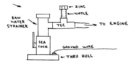
This arrangement provides zinc protection for the engine and makes it easy to inspect and replace the zinc. Also, instead of the small pencil zinc now provided, you can use a much larger zinc. A 3/4" bronze tee fit my strainer. On the subject of zincs, the Stennis' when at the dock connect a large zinc to their boat ground and hang it overboard -- good idea.
