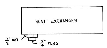
You hold onto the 7/8" hex with one wrench and unscrew the 3/4" plug. Mine was too corroded to move and it's too easy to tear the thin exchanger shell. Besides it was just about impossible to reach, The solution, suggested by the C, E. Smith Co., is to abandon the heat exchanger zinc and put one in a convenient easy to reach location like such
